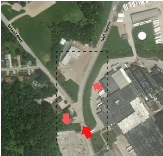
Figure 18: The gap in the levy causes it to be an insufficient measure against flash flooding from Geneva Creek.
