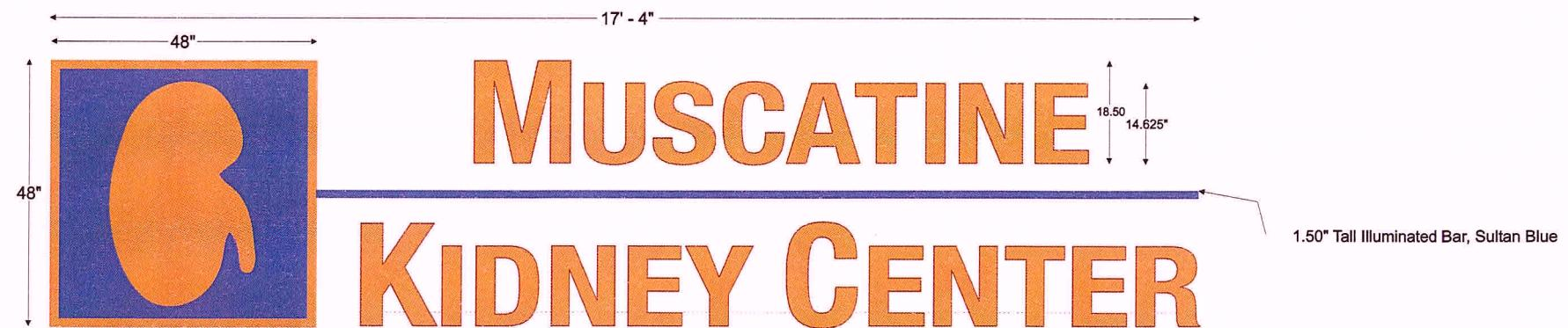
Illuminated Channel Letters Mounted On A Raceway
