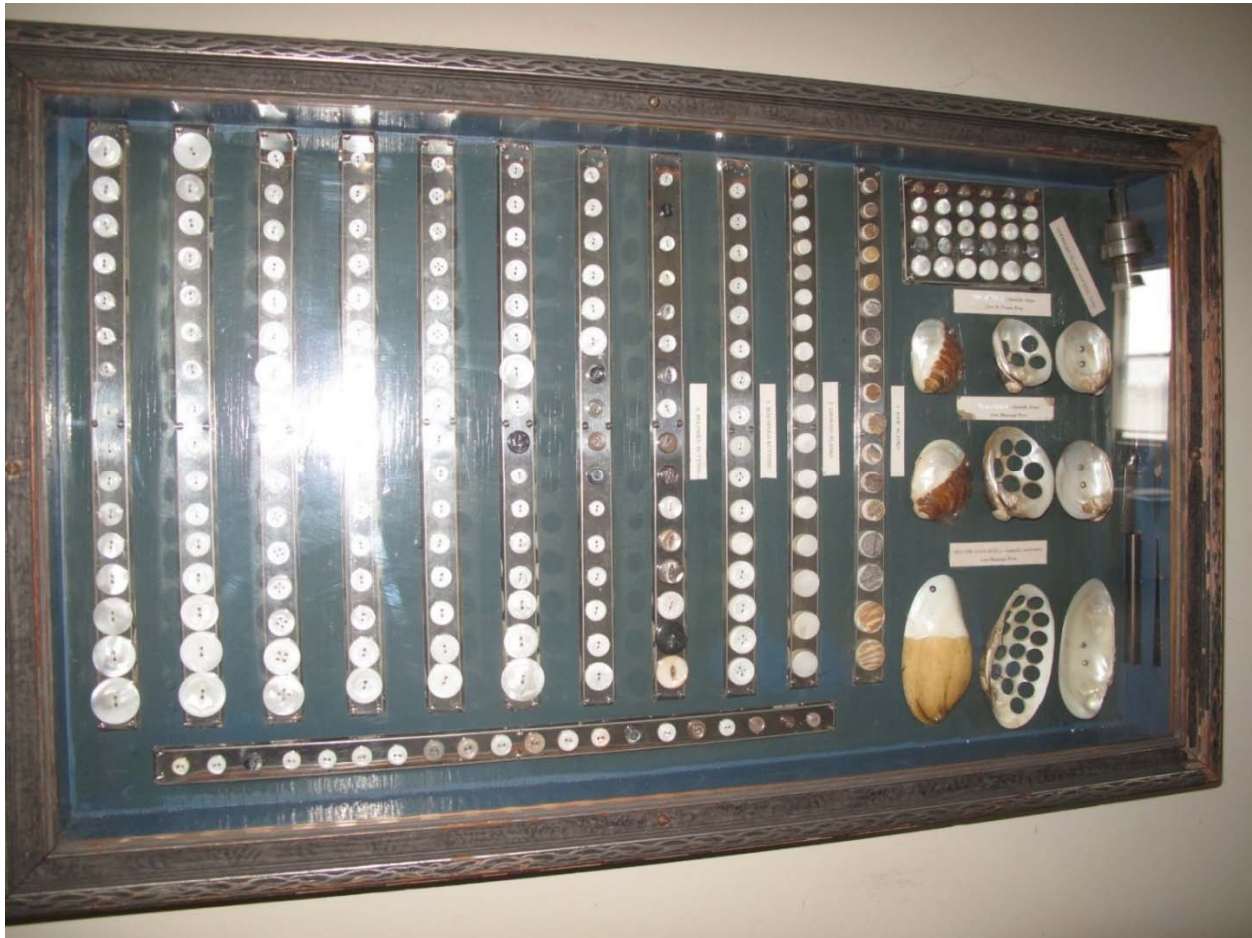
Figure 38. Display panel on freshwater pearl buttons, with production steps on right and variety of finished buttons on left (McKee collection).
