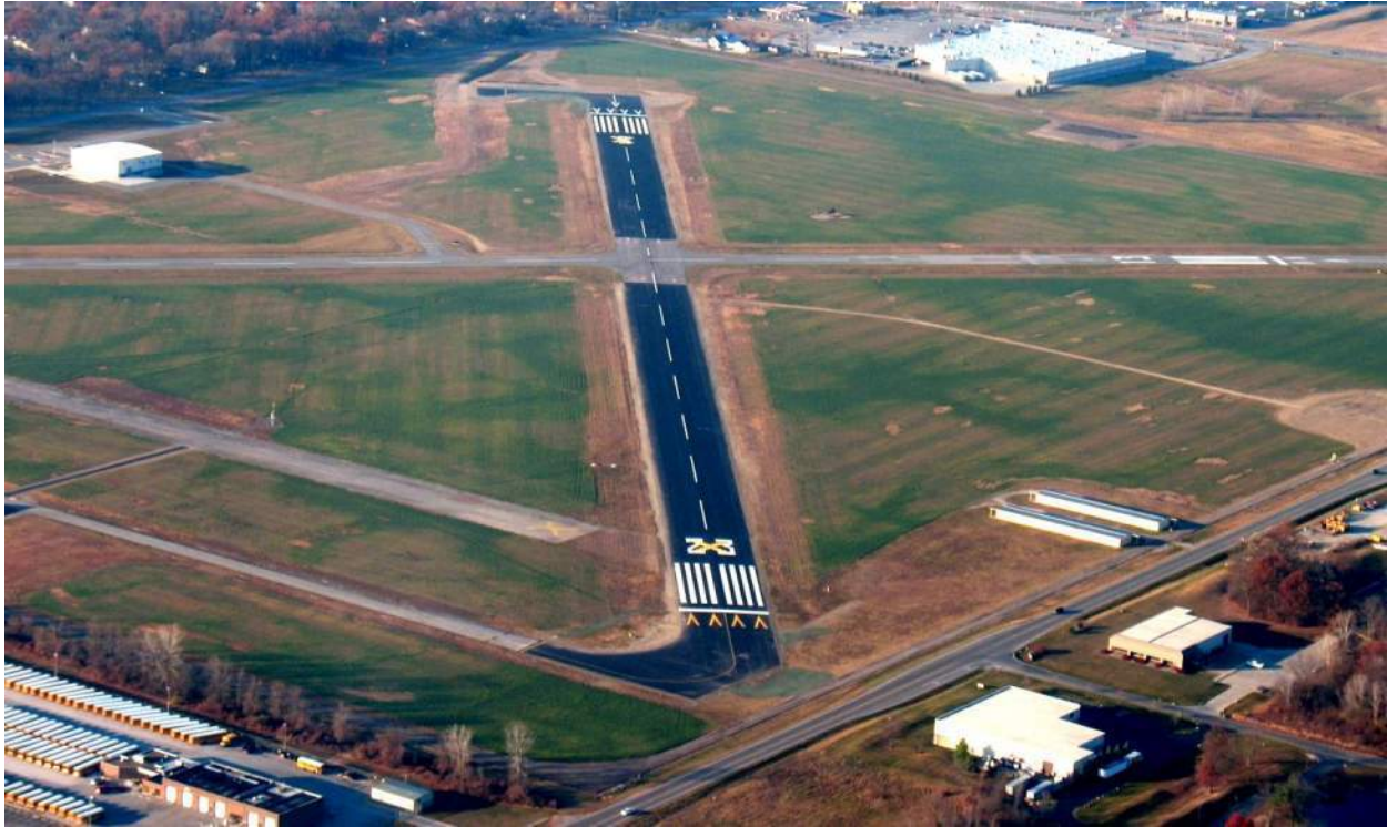
Figure 2-3. Markings for a Temporarily Closed Runway
